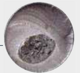
Analysis of the fracture surface following the fatigue strength test
