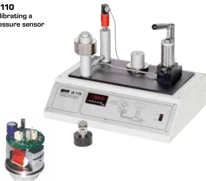
Interior layout of an electronic pressure sensor
