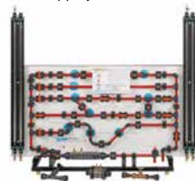
HM 150.11 Losses in a pipe system
