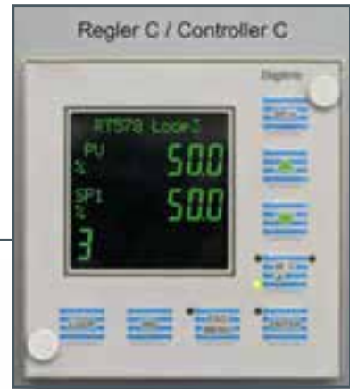
Digital controller The trainer uses an industrial compact controller for the instrumentation of single control loops. Internally, it has a total of four individual controllers, which can be used independently from each other.
