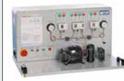
ET 180 Pressure switches in refrigeration
