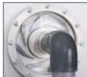
Vanes and impeller of the Francis turbine
