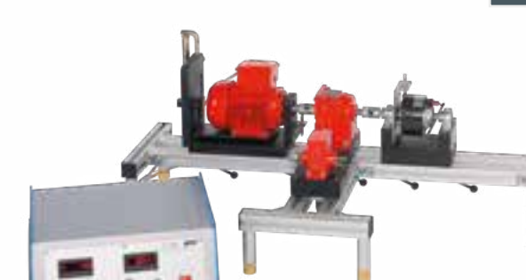
AT 200 Determination of gear efficiency
