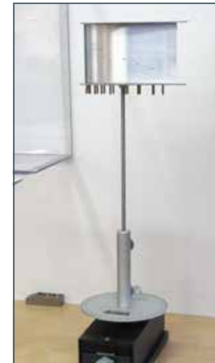
Pressure distribution on an aerofoil immersed in a flow
