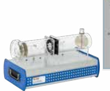
HM 282 Experiments with an axial fan
