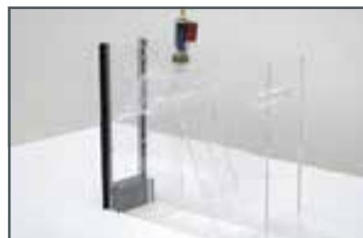
Siphon weir HM 160.36
