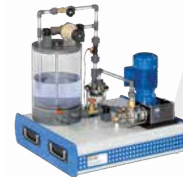
HM 285 Experiments with a piston pump
