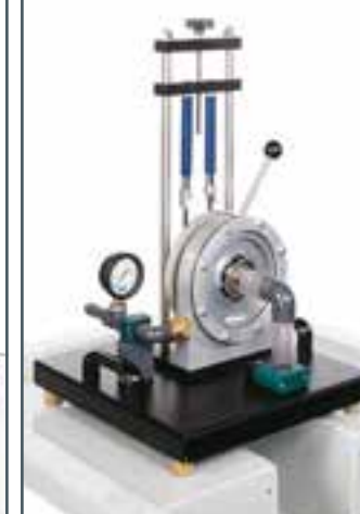
HM 150.20 Operating principle of a Francis turbine
