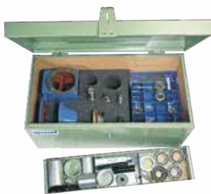
MT 110.02 Assembly spur wheel / worm gear mechanism
