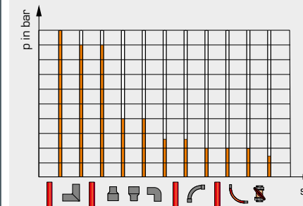
Sample measurement of the pressures between the various pipe elements
