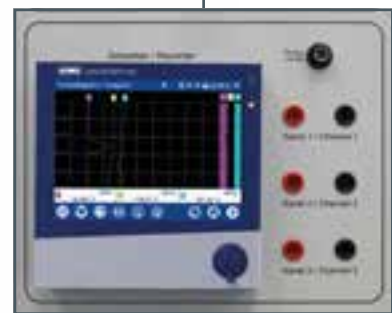
Digital recorder Three-channel paperless recorder to record the control processes.
