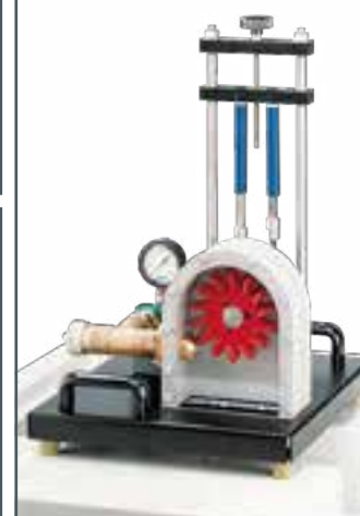
HM 150.19 Operating principle of a Pelton turbine
