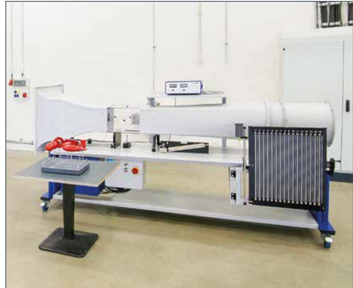
HM 170 with optional accessories: different drag bodies and HM 170.50 16 tube manometers
