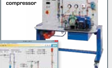
ET 432 Behaviour of a piston compressor
